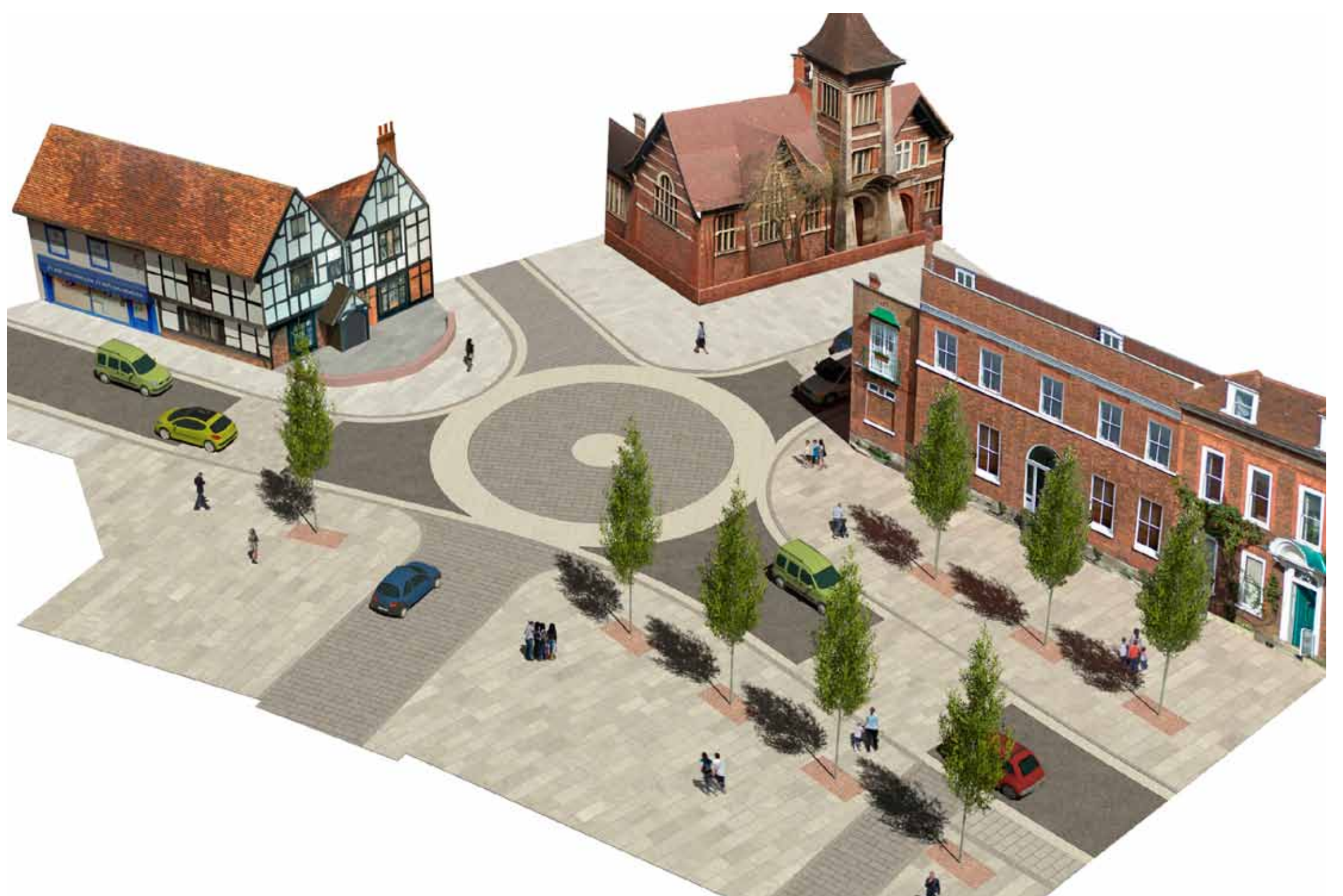
WHERE CONFLICTING STREAMS OF TRAFFIC INTERSECT A SIMPLIFIED APPROACH TO TRAFFIC MANAGEMENT IS POSSIBLE BASED UPON DESIGN PRINCIPLES THAT ENCOURAGE LOWER TRAFFIC SPEEDS
